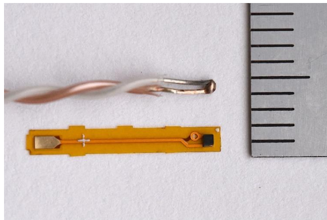
Figure 1. Single diode thermometer (bottom) compared to thermocouple (top), scale is in millimeters
