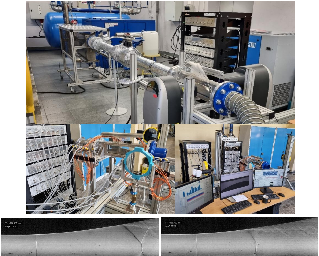
Figure 1. The view of the air system for the nozzle tests and the exemplary Schlieren photographs of the moist air flow through the nozzle
