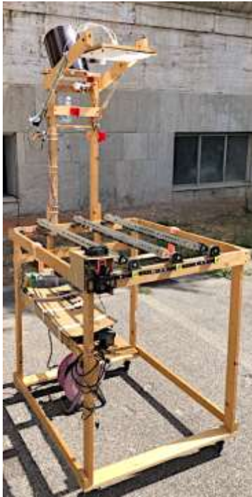
Figure 2. Lab-scale prototype of the BAF concentrator
