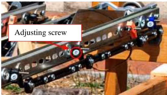
Figure 7. Mirrors' initial position adjustment system
