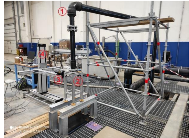
Fig. 1 Set-up for LDA measurement of the water speed. The following can be distinguished: 1 Supply pipe, 2 Pelton nozzle, 3 Laser emitter, 4 Drive traversing system.
