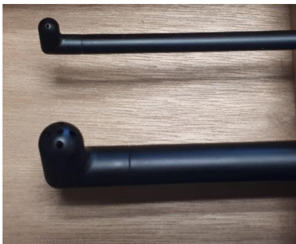
Figure 2 : the two probes used for the experiment. The heads were 3D printed and assembled with the masts in VKI.
