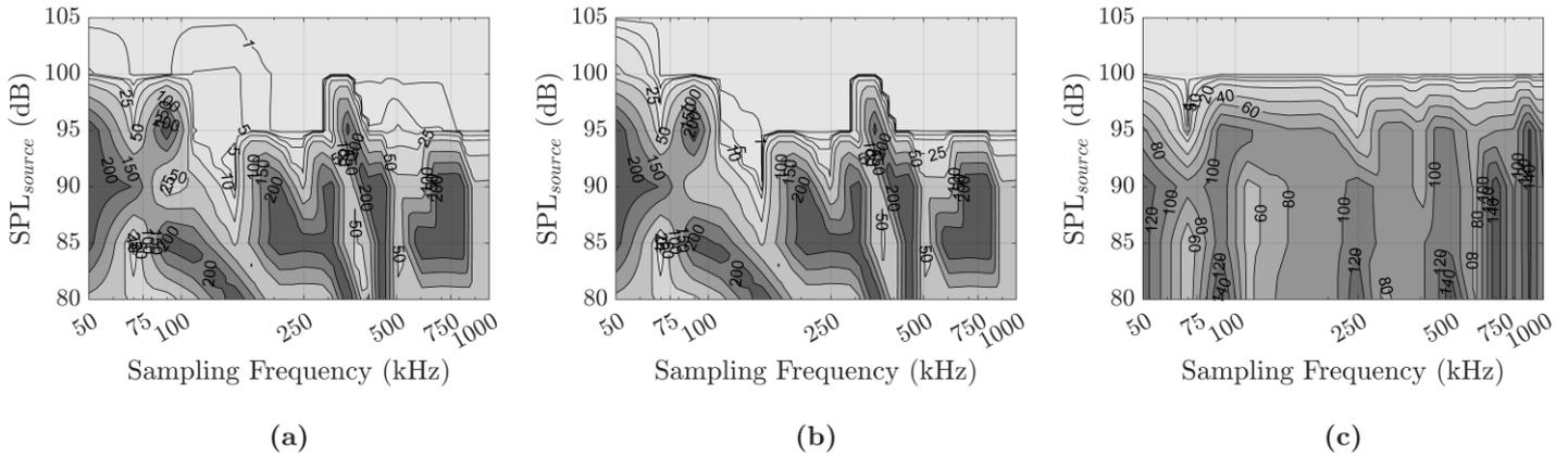
**FIGURE 7:** TOF ESTIMATION ERROR MAPS ( $SPL_{noise}=100$  dB;  $N_{tries}=1$ ): (a) PURE TONE; (b) LINEAR CHIRP; (c) WHITE NOISE
