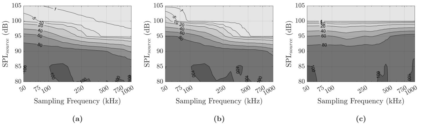
**FIGURE 8:** TOF ESTIMATION AVERAGE ERROR MAPS ( $SPL_{noise}=100$  dB;  $N_{tries}=1000$ ): (a) PURE TONE; (b) LINEAR CHIRP; (c) WHITE NOISE
