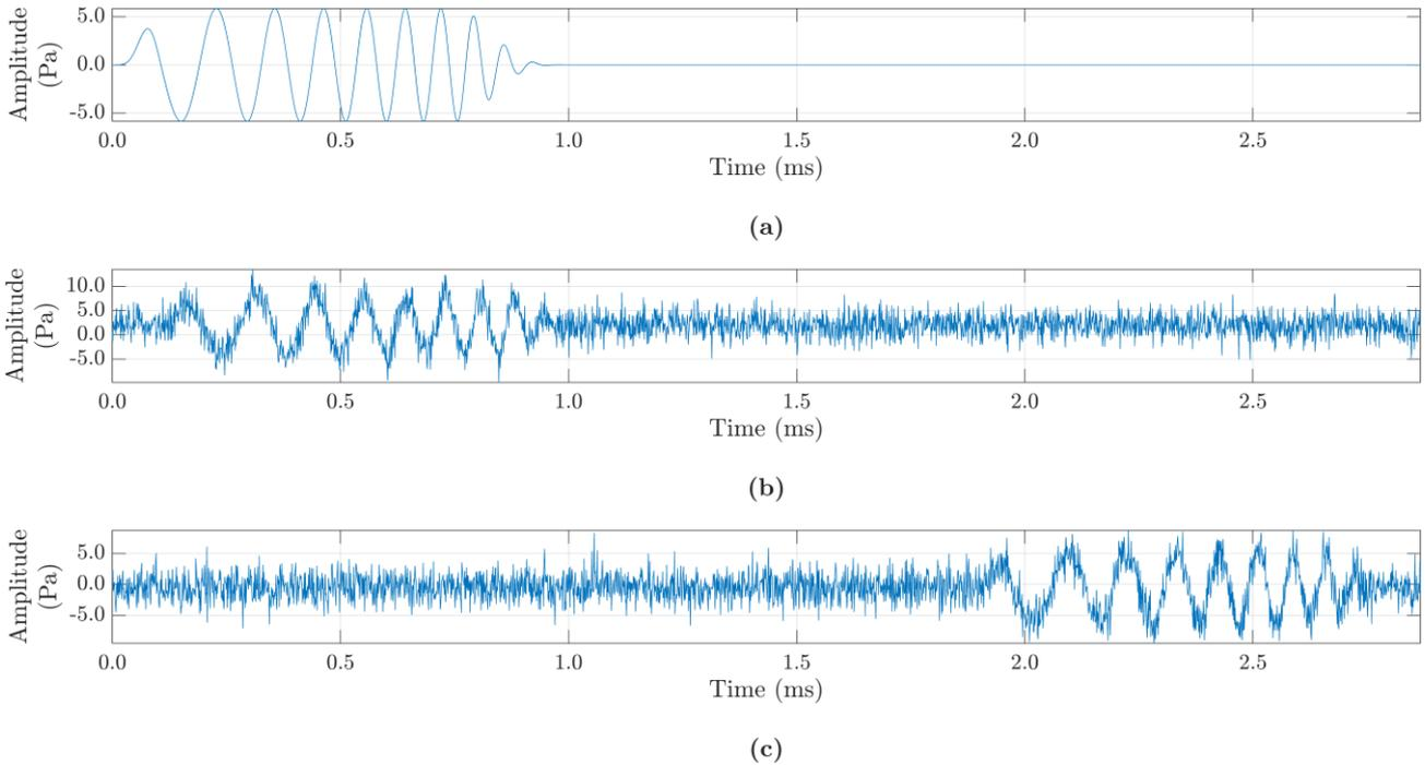
**FIGURE 5:** EXAMPLE OF LINEAR CHIRP SYNTHESIS: (a) SPEAKER; (b) FIST MICROPHONE; (c) SECOND MICROPHONE
