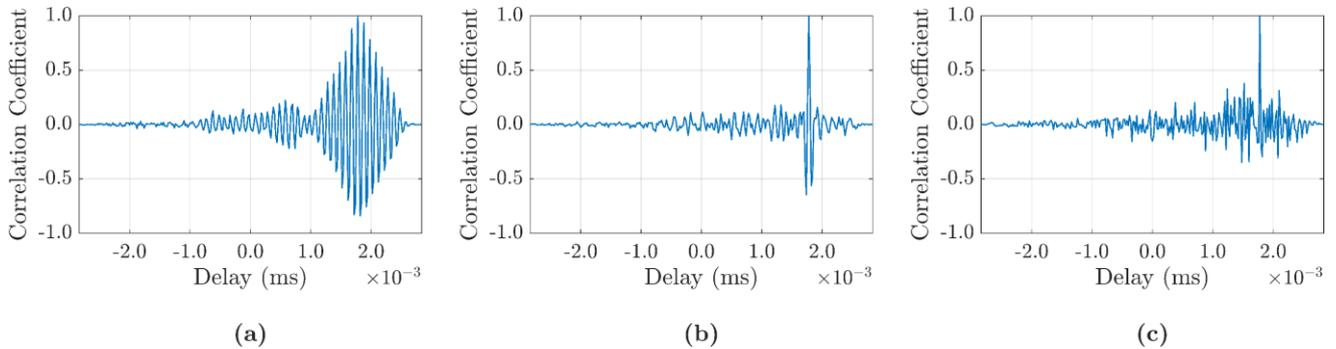
**FIGURE 6:** NORMALIZED CORRELATION COEFFICIENT: (a) PURE TONE; (b) LINEAR CHIRP; (c) WHITE NOISE
