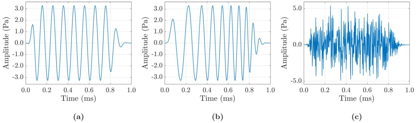
FIGURE 2: TEST SIGNALS: (a) PURE TONE; (b) LINEAR CHIRP; (c) WHITE NOISE
