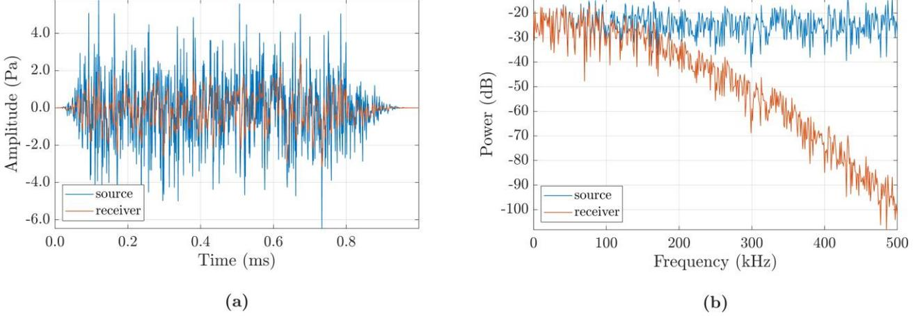
**FIGURE 4:** WHITE NOISE BEFORE AND AFTER SOUND ATTENUATION: (a) TIME DOMAIN REPRESENTATION; (b) POWER SPECTRUM
