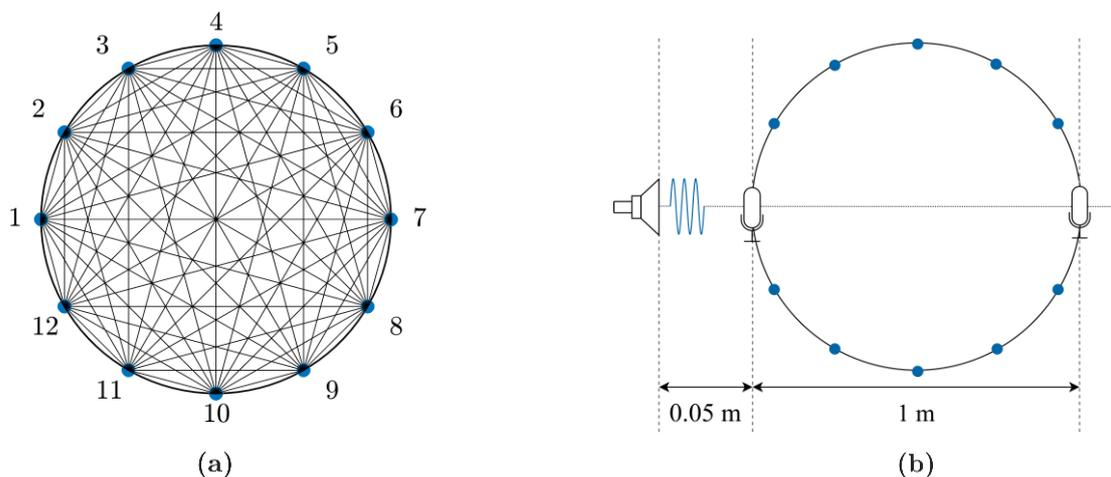
**FIGURE 1:** ACOUSTIC PYROMETER SET-UP: (a) ERCs DISPOSITION; (b) ERC SIMPLIFIED SCHEMATIC
