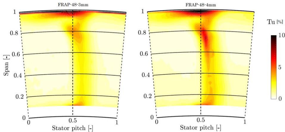
**Figure 1.** Turbulence at the exit of first stator with FRAP-4S 3mm (left) and 4mm tip diameter (right).
