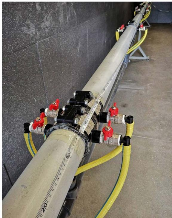
**Figure 1. Experimental setup for pipe leakage detection and localization**
