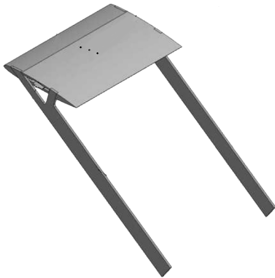
Figure 1: Model of airfoil with supporting stripes.
