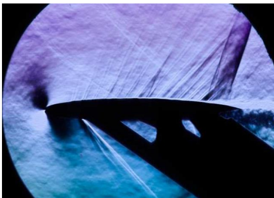
Figure 10: Schlieren picture taken at M_1 = 0.988 showing flow disturbances on the upper surface of the airfoil due to imperfect coverage of leadwires.
