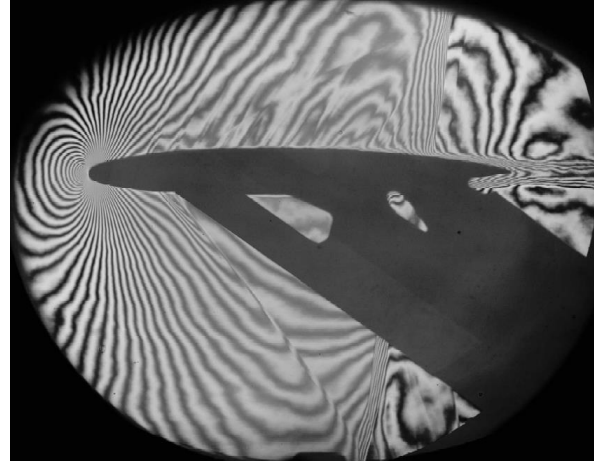
Figure 14: Interferograms taken at subsonic case M_1 = 0.75 (left) and transonic case M_1 = 0.97 (right) - cases with smooth leading edge.
