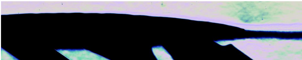
Figure 17: Schlieren visualization of the upper surface boundary layer in case with smooth leading edge. ( M_1 = 0.76 )
