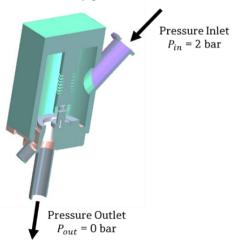
Figure 1: Control valve model
