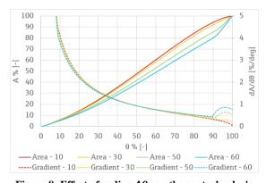
Figure 8: Effect of radius  $\Delta\theta_c$  on the control valve's characteristics
