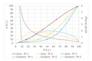
Figure 9: Effect of polynomial's order N on the control valve's characteristics
