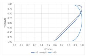
Figure 11: Effect of thickness on the flow profile 10D downstream the control valve
