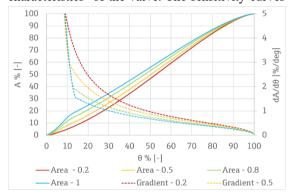
Figure 7: Effect of radius R<sub>1</sub> on the control valve's characteristics
