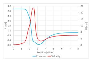
Figure 12: Pressure and velocity variation across the control valve
