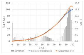
Figure 14: Percentagewise comparison of crosssectional area and mass flow of the control valve
