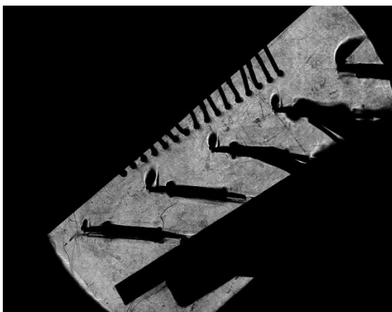
Figure 5. Shock Visualization (Ma=0.81)
