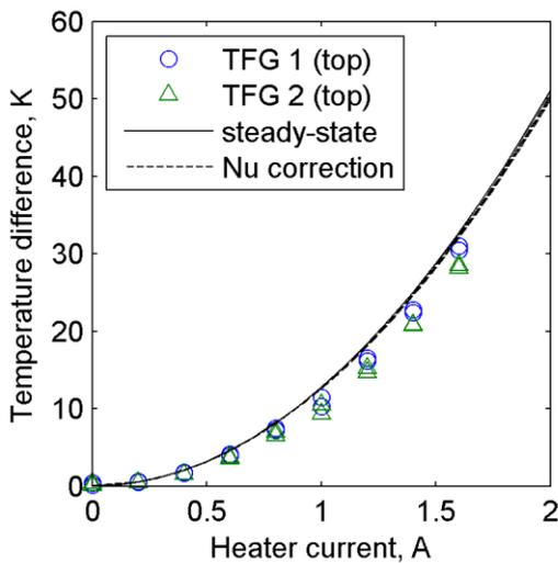
**Figure 5:** Preheating top gauge temperature differences over increasing heater current for 18 consecutive tests and comparison to analytical results.
