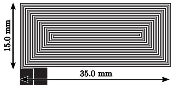
**Figure 4:** Example of a heater design.
