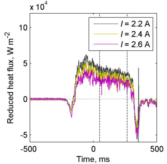
**Figure 7:** Heat flux traces for one double-sided gauge with an underside heater.
