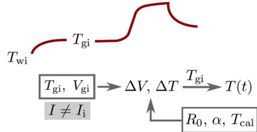
**Figure 9:** Principle of operation to measure the surface temperature history for self-heating thin film gauges.
