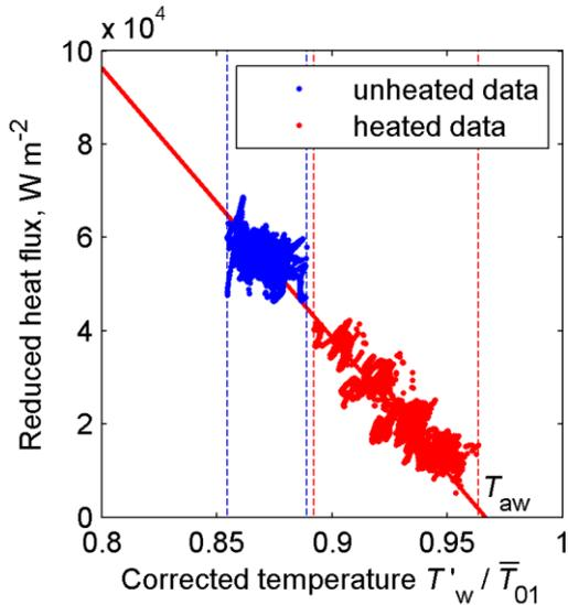
**Figure 14:** Regression data for one self-heating double-sided gauge compared to results from unheated double-sided thin film gauges.
