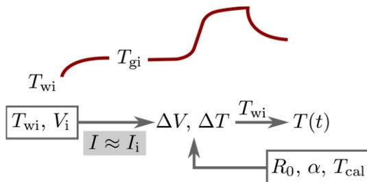
**Figure 2:** Principle of operation to measure the surface temperature history for a heated thin film gauge arrangement with a separate heating system.
