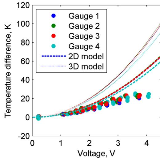
**Figure 12:** Bottom gauge temperature difference for different gauge settings plotted over voltage across the top gauge and superimposed to the 2D and 3D thermal conduction model results.
