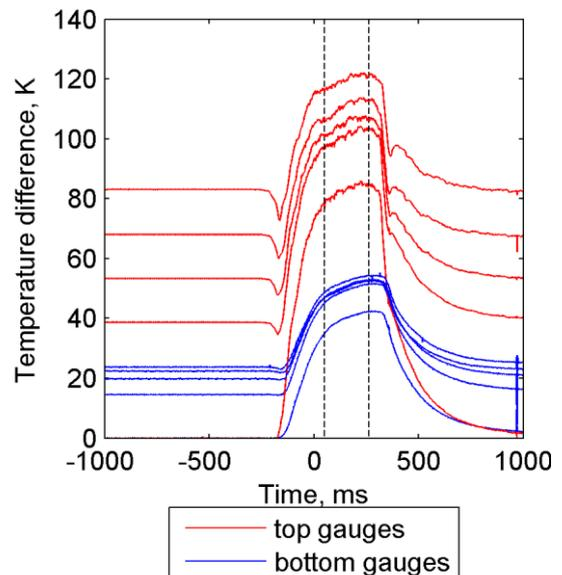
**Figure 13:** Temperature traces for one self-heating gauge (one unheated run and four heated runs).
