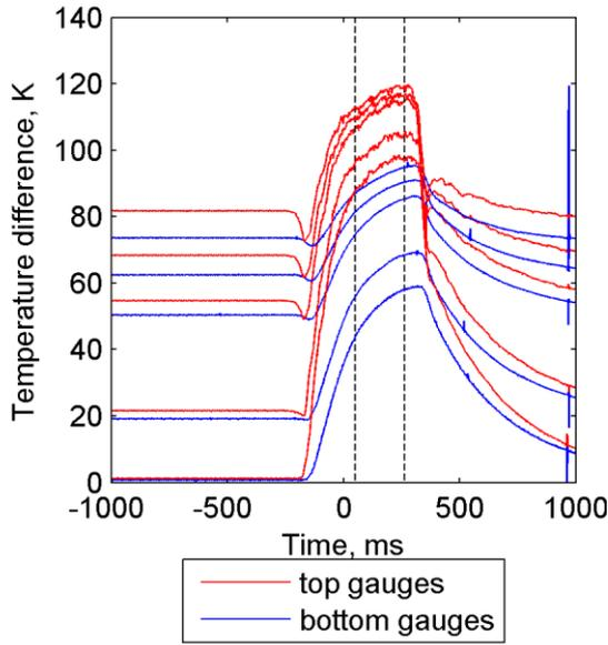
**Figure 6:** Temperature traces for one double-side gauge with an underside thin film heater (one unheated run and four heated runs).
