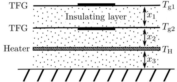
**Figure 3:** Heated thin film gauge arrangement with an underside thin film heater.
