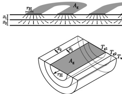
**Figure 11:** Representation of the gauge geometry (see Figure 1 and 10) with a 2D conduction model.
