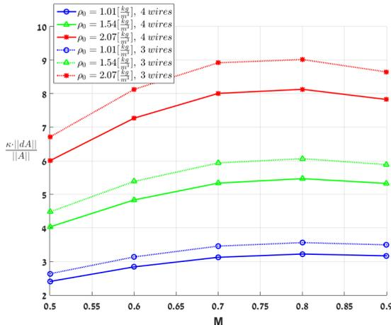
Figure 7 – Contrasting the error amplification due to sensitivity matrix perturbation for best 4-wire and 3-wire probes, Value function 4 at  $T_0 = 350K$
