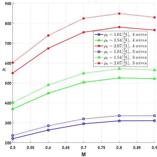
Figure 6 – Contrasting the Condition numbers of best 4-wire and 3-wire probes for Value function 4 at  $T_0 = 350K$
