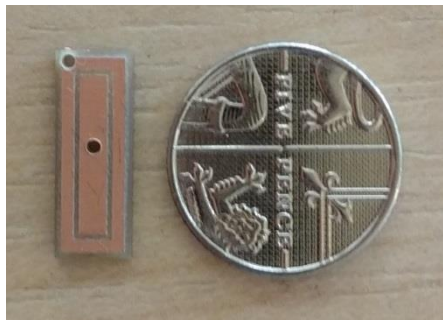
Figure 6 – Sensor after CNC manufacture.
