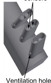
Figure 2: detailed view of the measuring heads. Adapted from Lahalle [1].
