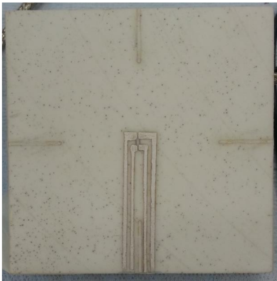
Figure 6: The MACOR impingement plate before painting with high-emissivity high-temperature paint.
