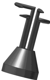
Fig. 1b. 120 deg, Z-type DHW probe without wake interference effects.
