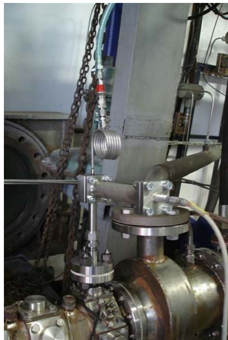
Fig. 6: New-design microphone probe during the high pressure test at COMOTI, Romania
