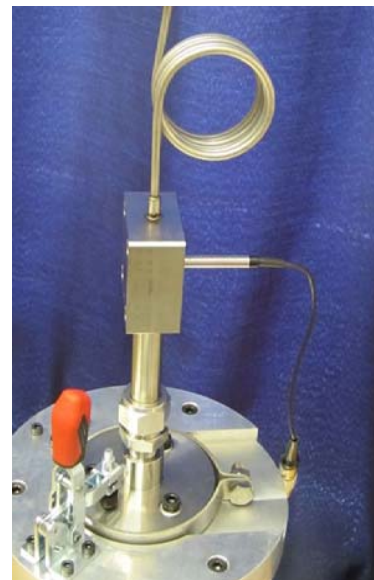
Fig. 2: Microphone and pre-amplifier are mounted perpendicular to the connection tube.
