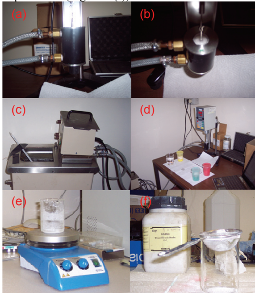
Figure 8: The viscosity measuring system: spindle/chamber/heat exchanger (a-b), water bath of the heat exchanger (c), viscometer layout (d), magnetic mixer (e), \text{TiO}_2 (f)
