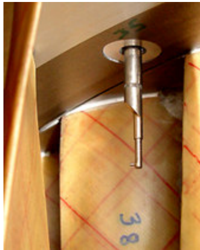
Fig. 6 Unsteady total pressure probe installed in an axial research compressor.
