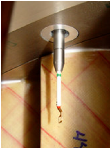
Fig. 5 Split-fiber probe in the gap between the rotor and stator of the compressor first stage.
