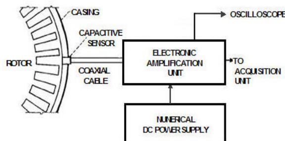
Figure 4. Acquisition chain diagram
