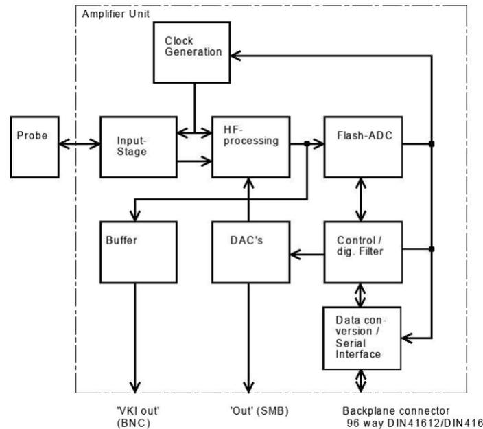
Figure 6. Diagram of the amplification unit
