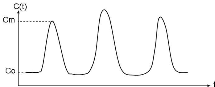
Figure 2. Capacity variations due to a blade passing
