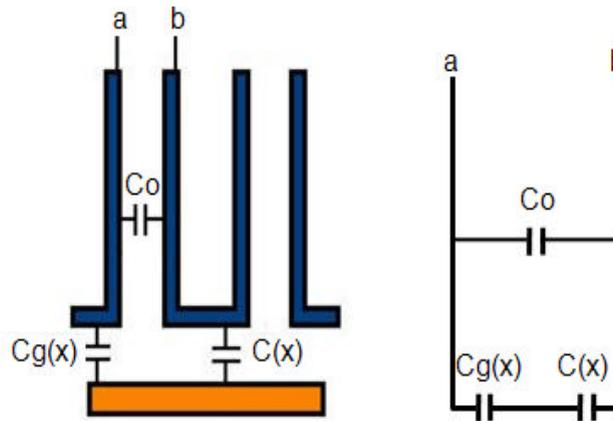
Figure 1. Working principle of the capacitive probe
