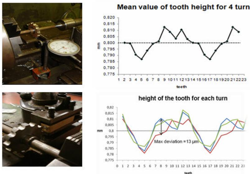
Figure 16. Mechanical measurement results versus capacitive probe results
