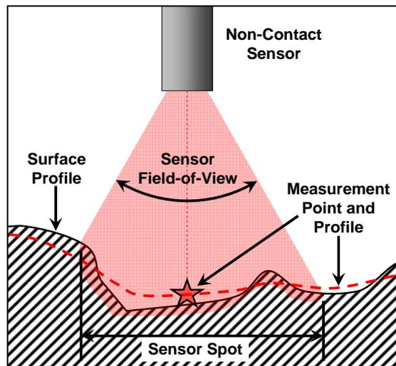
Figure 3. Illustration showing spatial filtering effect on non-contact measurements
