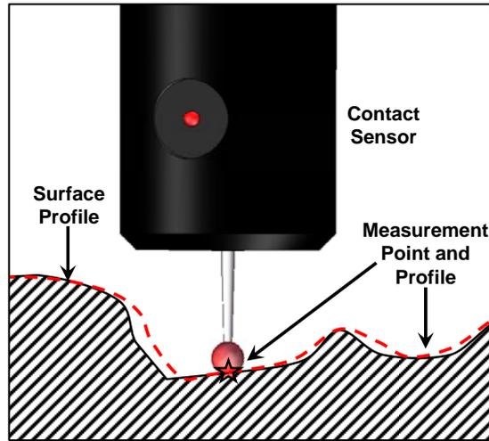
Figure 2. Illustration showing ruby-tipped touch probe and the resulting spatial filtering of contact measurements
