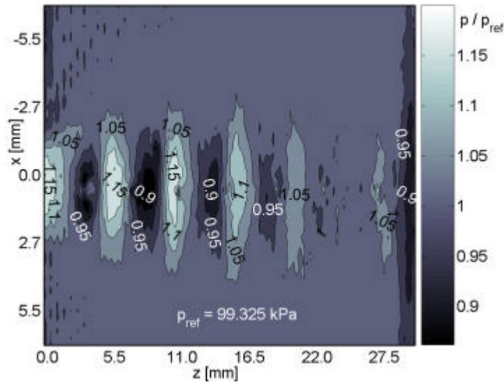
Figure 13: Pressure distribution obtained by PSP, impinging under-expanded jet,  $D_p = 3$  bar
