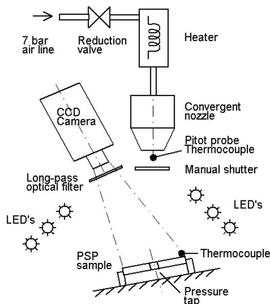
Figure 6: Temperature step test – intermittent hot jet
