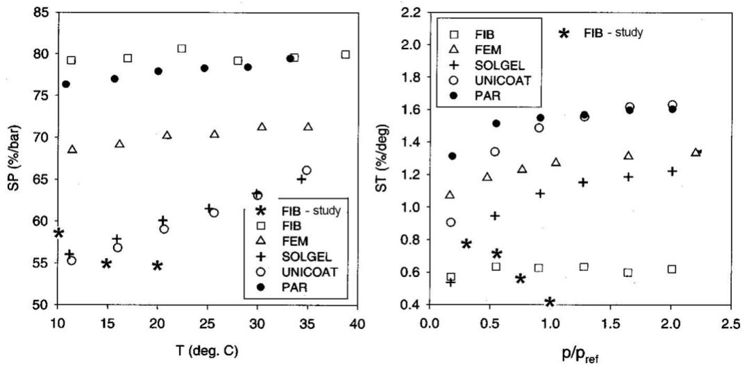
Figure 3: Comparison of pressure and temperature sensitivity from Lachendro (2000), study data added (PtTFPP in five different polymer binders; P<sub>ref</sub> = 1 bar, T<sub>ref</sub> = 283 K)
