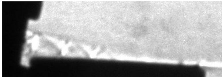
**Figure 12: Shadowgraph of impinging under-expanded jet,  $Dp = 3$  bar**
