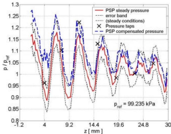
Figure 14: Comparison of pressure distribution along the plate axis, impinging under-expanded jet,  $D_p = 3$  bar
