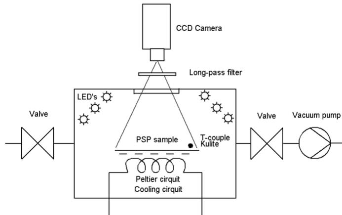
Figure 2: Steady-state calibration setup
