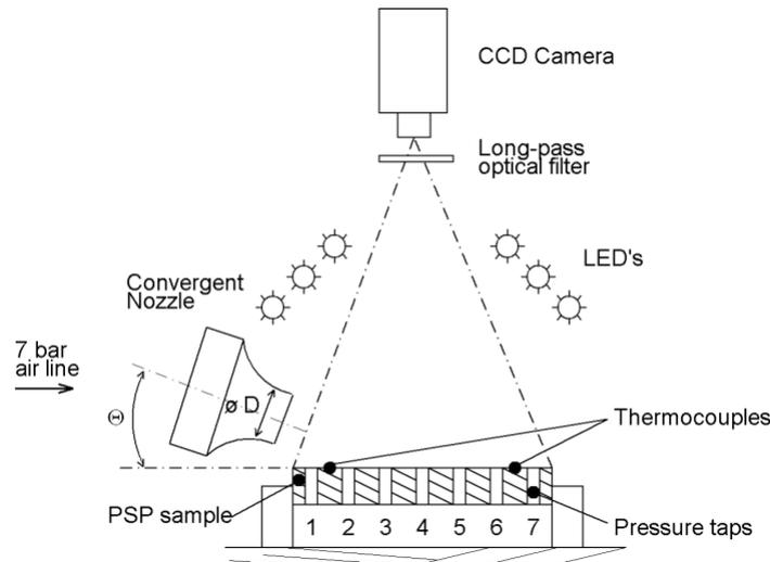
**Figure 11: Scheme of impinging jet arrangement**
