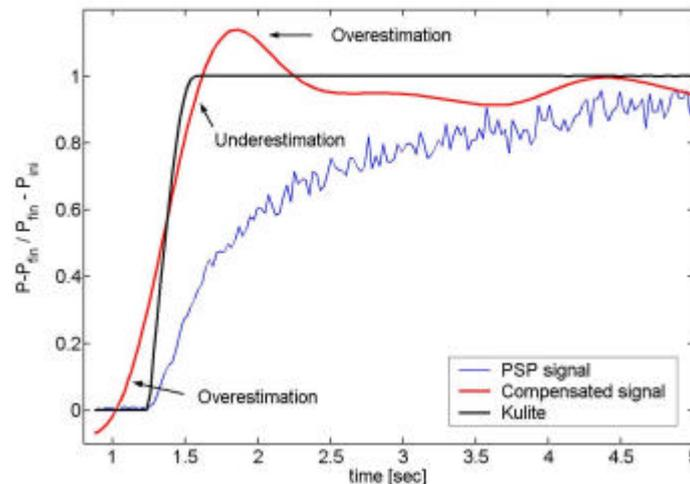
Figure 10: Compensated signal by linear differential eq., 5<sup>th</sup> order, 1 step delay
