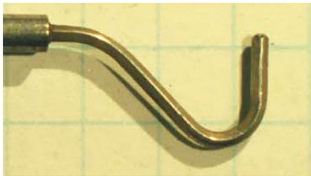
Figure 2: Cobra-Head Pneumatic Five-Hole Probe
