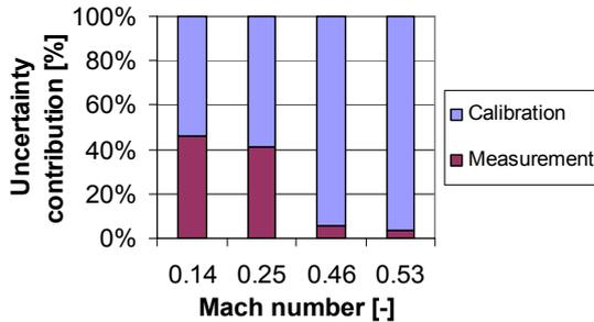
Figure 8: Uncertainty contribution of calibration and measurement of four Mach numbers [-] (using Calibration polynoms)
