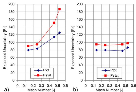
Figure 13: Expanded uncertainty ( $k=2$ ) of the total pressure and static pressure derived with a) Calibration Polynoms b) Look-up tables
