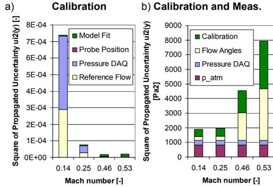
Figure 12: Square of propagated uncertainties  $u_i^2(y)$  of 4 Mach numbers a) Calibration  $\Delta Kt^2$  [-] b) Calibration and Measurement  $\Delta Pt^2$  [ $Pa^2$ ] (using Calibration polynoms)
