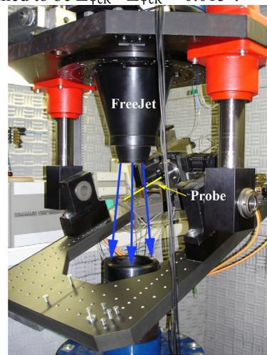
Figure 4: Freejet Probe Calibration Facility
