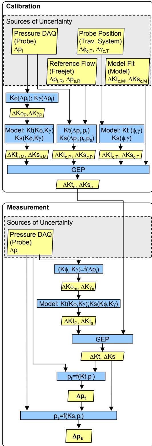
Figure 14: Uncertainty propagation of total and static pressure measurement – Method B
