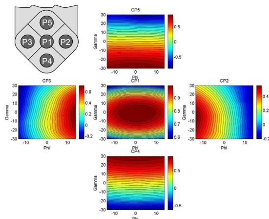
Figure 3: Pressure coefficient contours of a five-hole probe at  $Ma=0.25$
