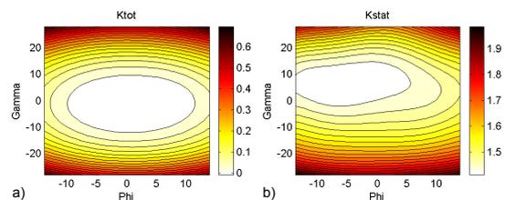
Figure 10: Distribution of calibration coefficients with respect to yaw and pitch angles at  $Ma=0.25$ , a)  $K_t$ , b)  $K_s$
