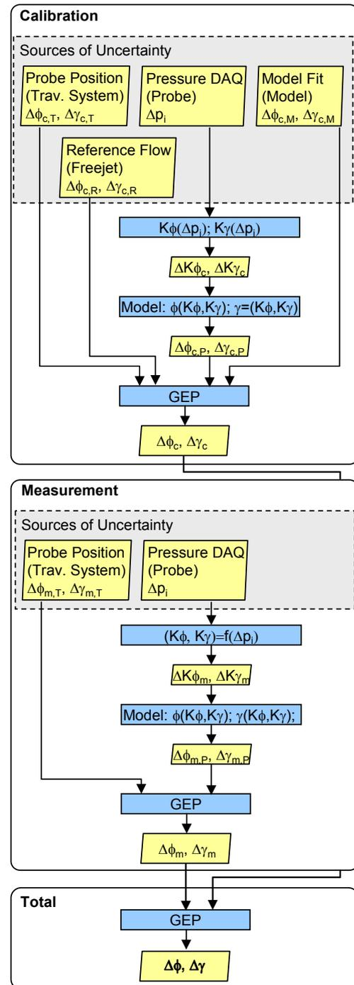
Figure 5: Uncertainty propagation of flow angle measurement
