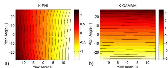
Figure 6: Distribution of calibration coefficients with respect to yaw and pitch angles at  $Ma=0.25$ , a)  $K\phi$ , b)  $K\gamma$
