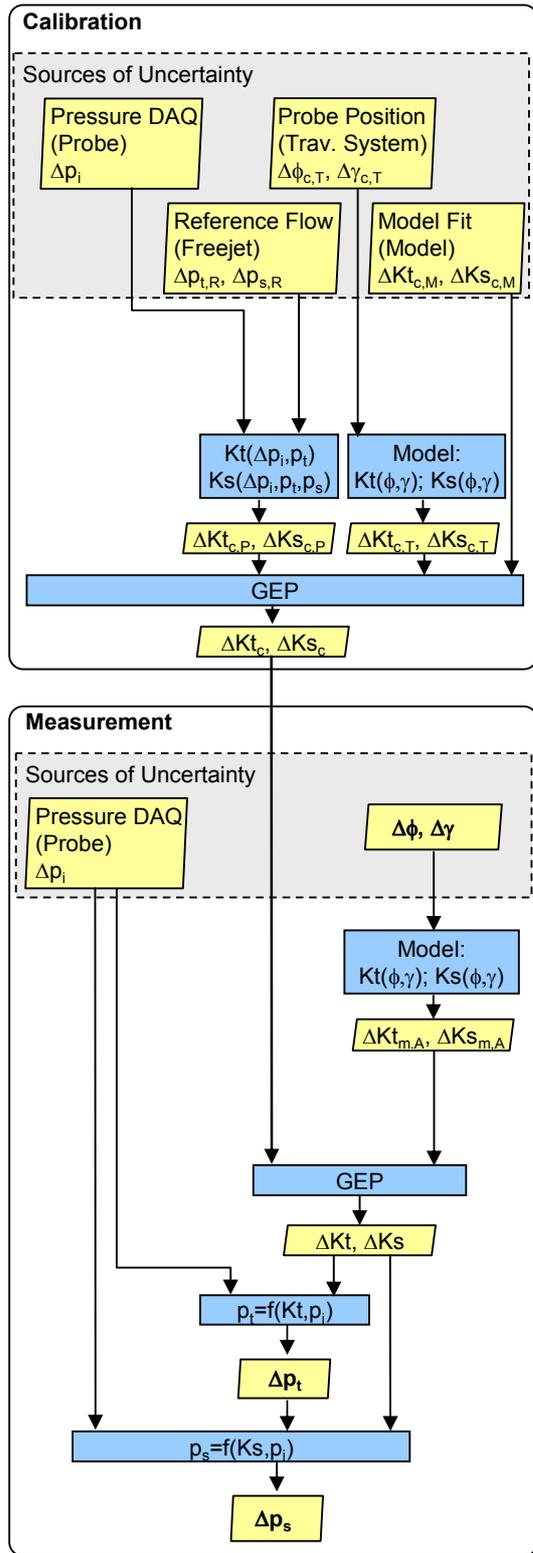
Figure 11: Uncertainty propagation of total and static pressure measurement – Method A
