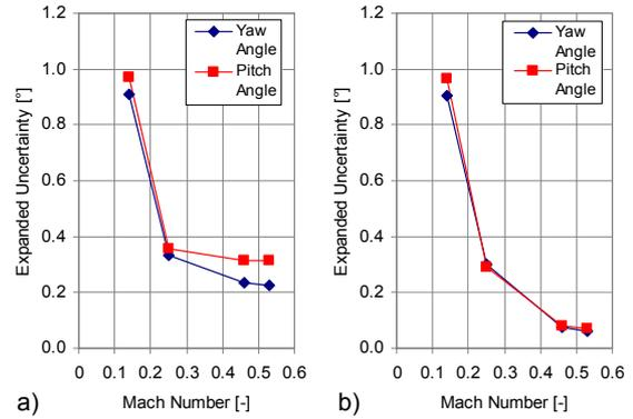
Figure 9: Expanded uncertainty ( $k=2$ ) of the yaw and pitch angle derived with a) Calibration Polynoms b) Look-up tables
