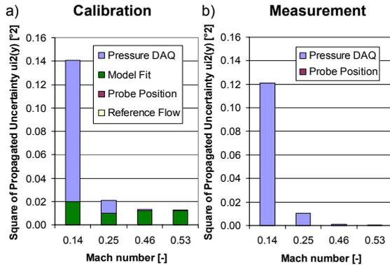
Figure 7: Square of propagated uncertainties  $u_i^2(y)$  [ $^{\circ 2}$ ] of four Mach numbers [-] a) Calibration b) Measurement (using Calibration polynoms)
