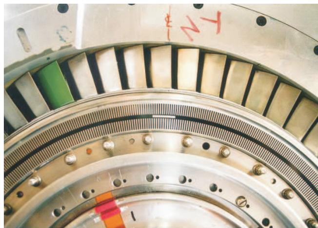
Figure 6. Detail of the printed encoder
