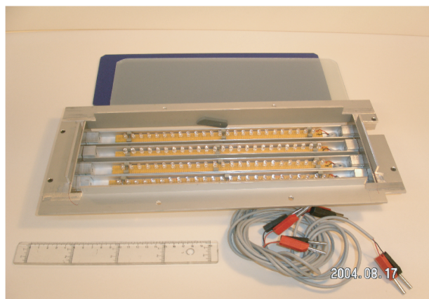
Fig. 3 LED-panel light source showing 4 rows of 25 diodes in each.
