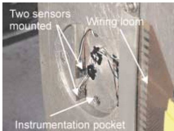
Figure 10: Close-up view of instrumentation pocket, showing two sensors mounted
