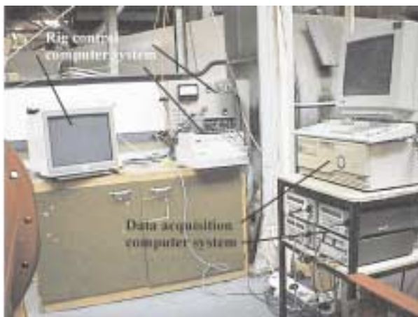
Figure 8: Spinning rig control and data acquisition system
