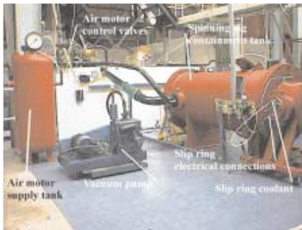
Figure 7: Spinning rig ancillary circuits
