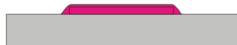
Figure 14 Cross section view after the etching of the second layer of PSG
