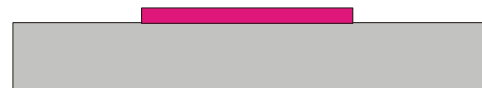
Figure 13 Cross section view after the etching of the first layer of PSG.
