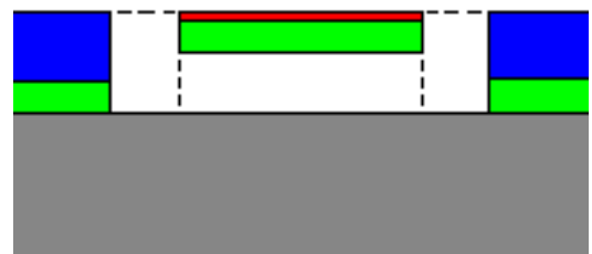
Figure 2 Schematic cross-section of the bridge (green) with the hot film (red) and the air gap around the bridge. Not to scale
