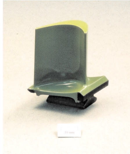
Figure 4b: A photograph of the turbine blade after application of the enamel coating
