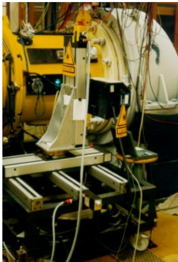
Fig. 5: 3D-L2F in front of test section and iced diffusion chamber on right hand side
