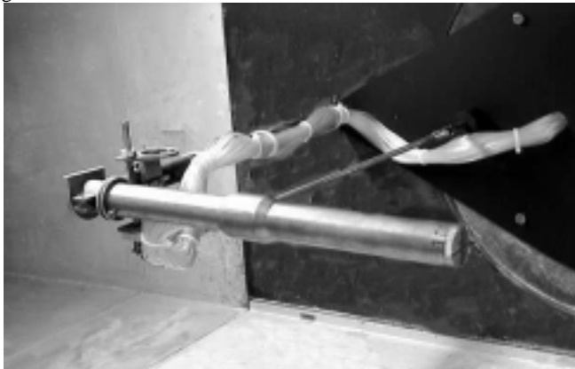
Fig. 4 Probe mounted in a low-speed wind tunnel
