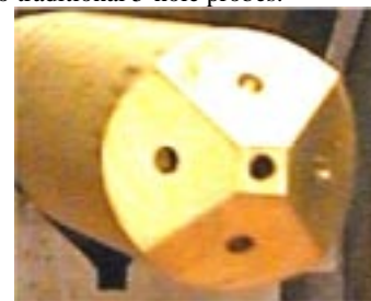
Fig. 18 Conventional 90° pyramid 5-hole probe
