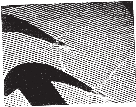
Fig.8 Real time shock visualisation using a carrier fringe system perpendicular to the shear direction (differential interferometry)
