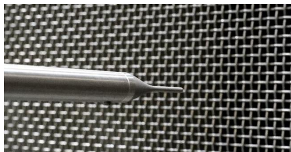
Figure 1. Wind tunnel set-up with the FRAP being installed downstream of the grid in the nozzle section.
