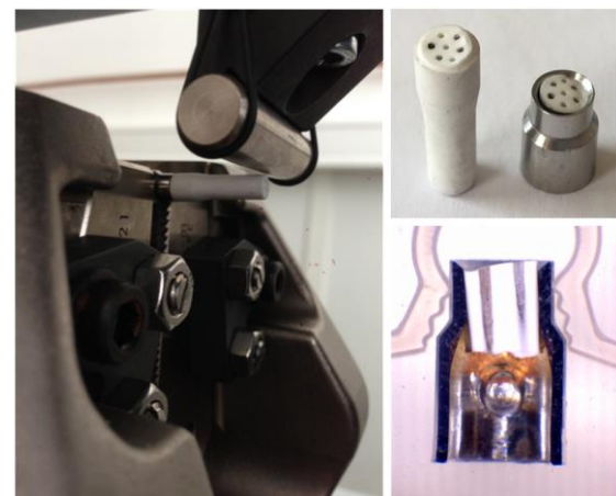
Figure 15: UHT Probe demonstrator mechanical testing
