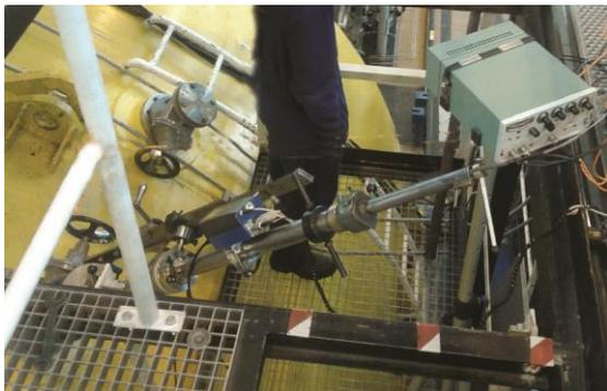
Figure 4: Rotating probe carrier with the anemometer
