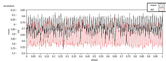
Figure 10: Phase-averaged signal, one revolution, in front of the last stage ( $r = 310$  mm)
