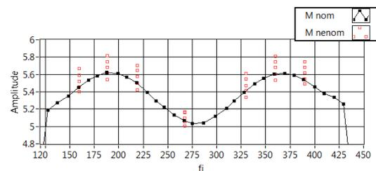
Figure 7: Example of the rotating probe record. The output voltage at the nominal wire temperature (black) and at additional temperatures (red)
