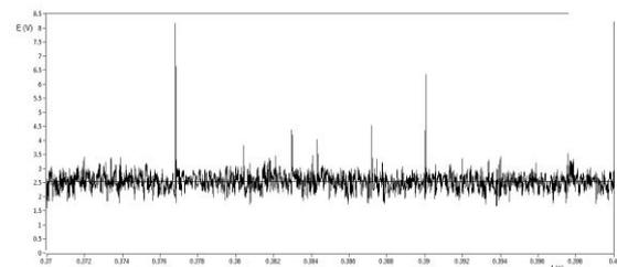
Figure 6: Anemometer signal of steam flow with water droplets
