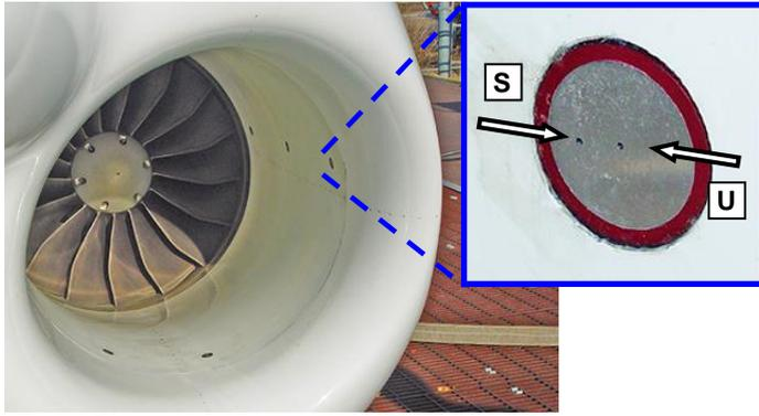
Figure 8: View of instrumented access ports
