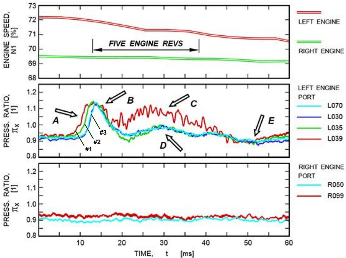
Figure 14: Left engine single stall event (0.06 s segment)
