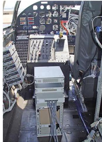
Figure 11: On-board main data acquisition unit
