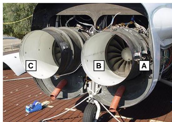
Figure 6: Instrumented engine intakes
