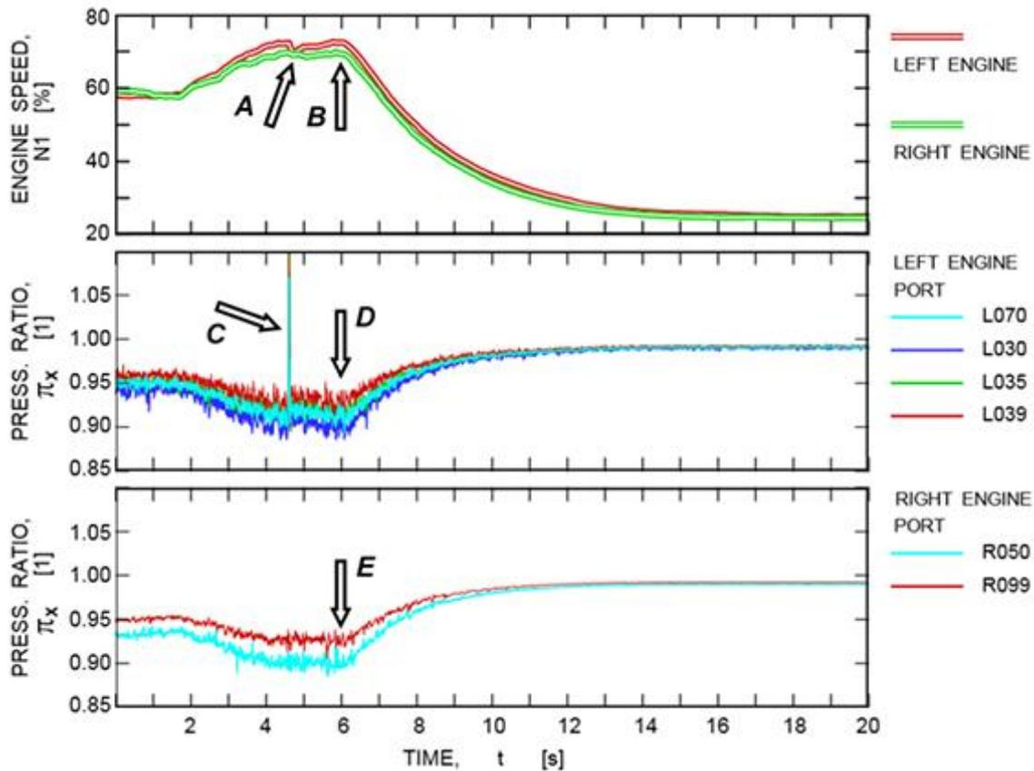
Figure 12: Left engine single stall event (20.0 s segment)
