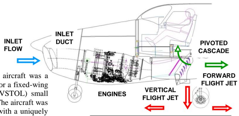
Figure 3: Thrust vectoring device
