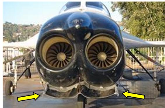
Figure 19: Double scoop flow deflector
