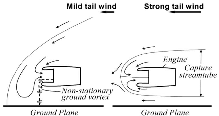
Figure 24: Effects of tail wind strength on ground vortex formation.
