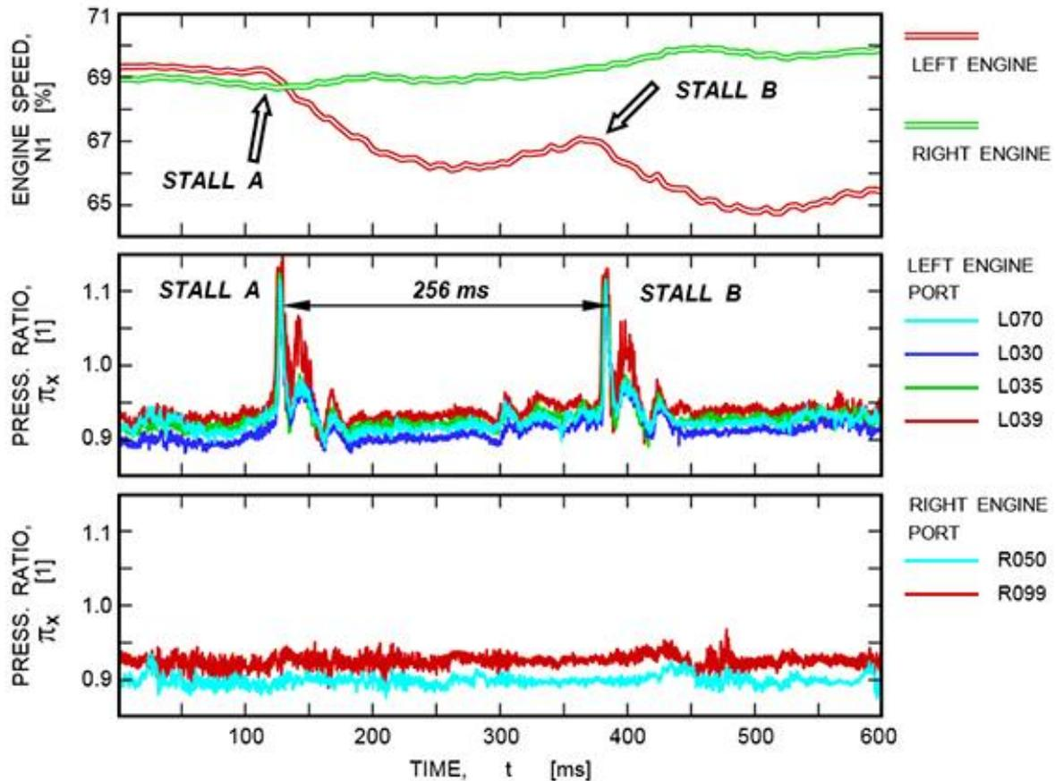
Figure 17: Left engine double stall event (0.6 s segment)
