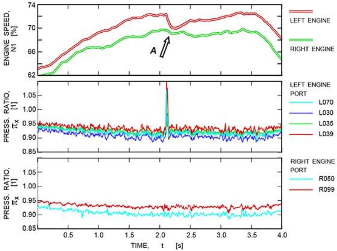
Figure 13: Left engine single stall event (4.0 s segment)
