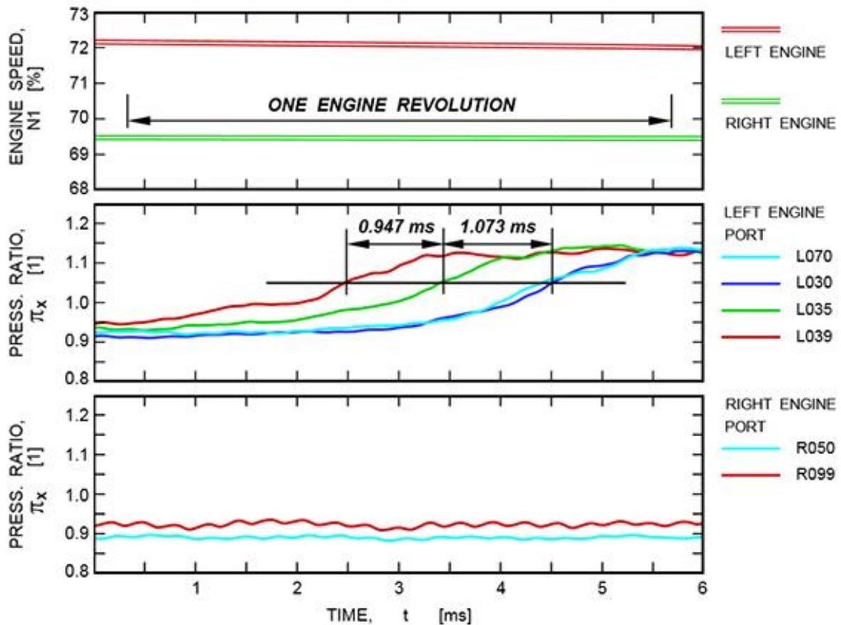
Figure 15: Left engine single stall event (0.006 s segment)
