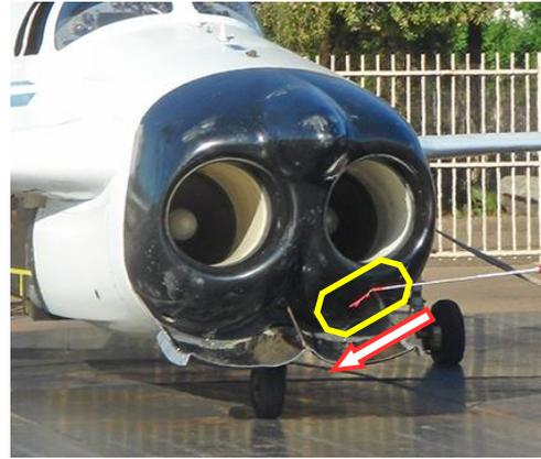
Figure 22: Prevailing flow at inlet lip level; scoop flow deflector deployed
