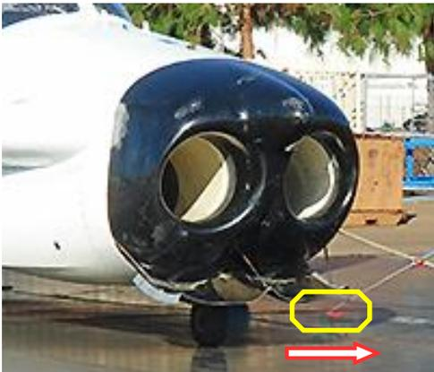
Figure 21: Prevailing flow at ground level; scoop flow deflector deployed
