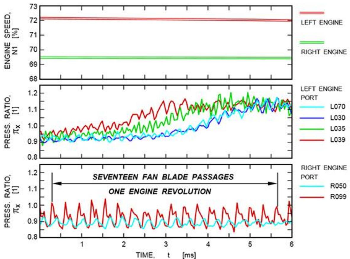
Figure 16: Left engine single stall event; unfiltered data (0.006 s segment)
