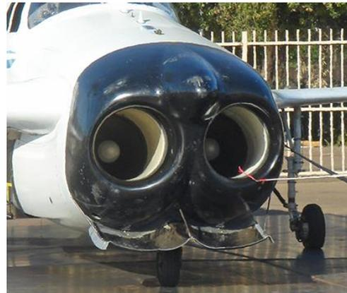
Figure 23: Prevailing flow at inlet mid level; scoop flow deflector deployed
