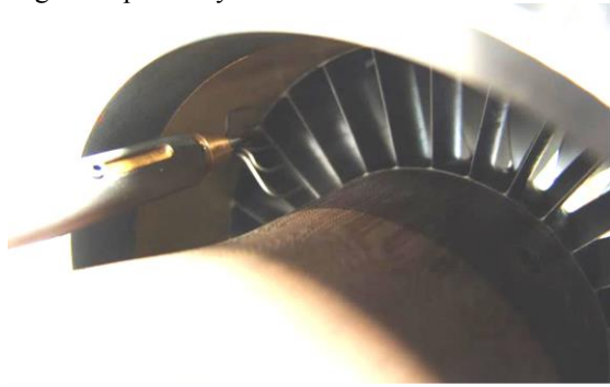
Figure 3: TPS fan OGV's and rotating rake head in rear axial position
