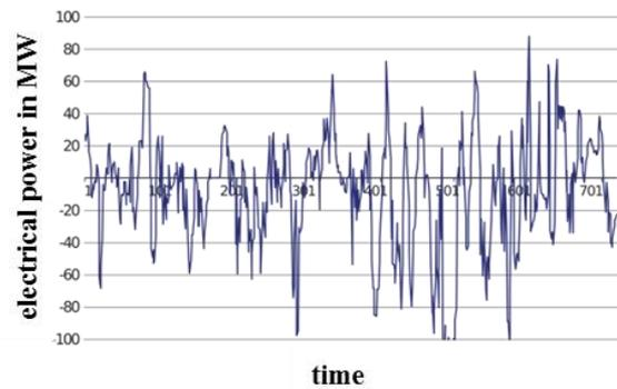
Figure 2: Hourly difference of predicted and actual power of the 160 MW offshore wind farm Horns Rev 1 (EURELECTRIC 2011)
